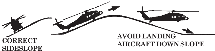
Figure 4-3. Determining Ground Slope
